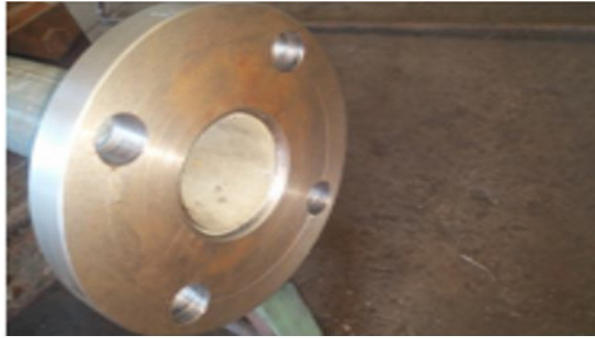
Figure 13.0 (2" 150 RF Screwed Flange to Parent Pipe fit up)
