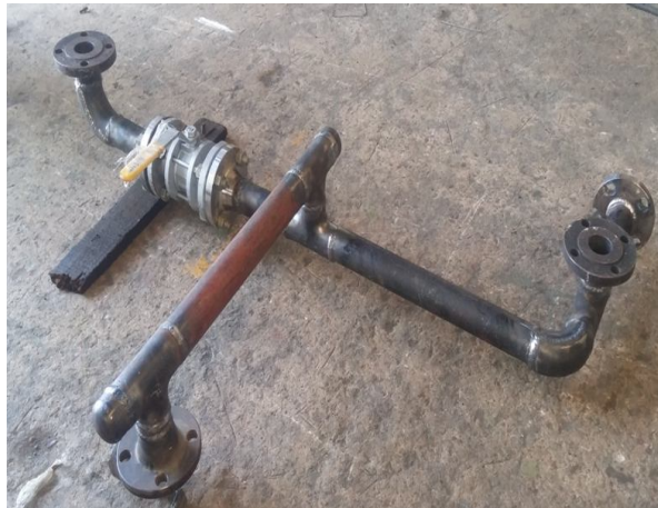
Figure 10.0 Prefabricated Loop S as Per New Design Concept Eliminating the Elbow Prone to Erosion
