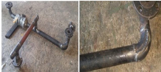
Fig 14.0 Newly developed design system to overcome the erosion in Drain network System
