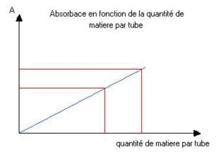
After obtaining the absorbance values of the calibration range, the absorption curve can be drawn OD=f(Quantity). A straight line must pass through the landmark origin and be as close as possible to most calibration points. The absorbance value of the test is plotted on this line to determine the amount of compound present. In order to find the concentration of the test compound present in the initial medium, the volume of the test sample and any dilution shall be taken into account.
