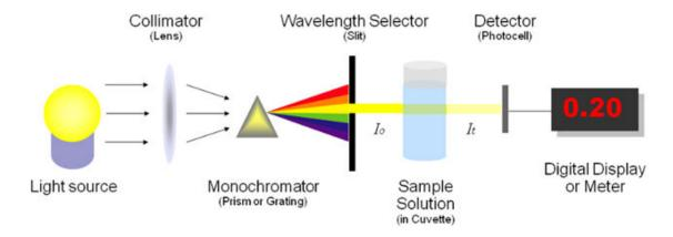
Basic structure of spectrophotometers
